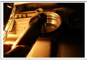
2. Remove the tool and check the bore with your little finger and try to remove any residual chips. You can plug the bore with your finger and blow out the rest of the cavity.
